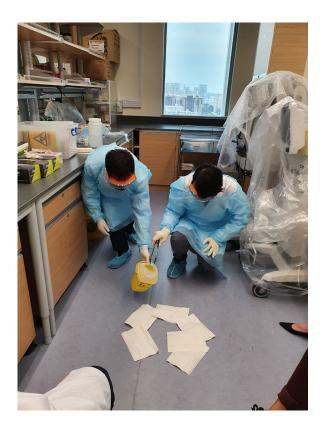
Participants removing sharps and disposing into the sharps bin during the simulated biological spill response cleanup
